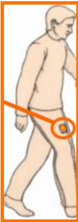
Figure 5: Typical placement of an inclinometer which is able to differentiate standing and sitting time
